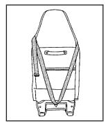
If the position you are using has an integrated headrest and you are using a dual tether, route the tether around the headrest.
